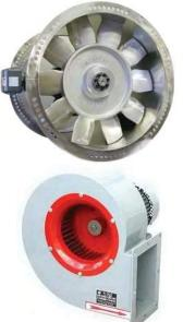
Axial-flow fans: Air passes through the fan parallel to the driveshaft. An axial-flow fan is suitable for a larger flow rate (CFM) with relatively small pressure gain. The effective progress of the air is straight through the impeller at a constant distance from the axis. These fans are widely used for providing the required airflow in heat and mass transfer operations.
