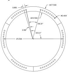
304 SS Laser cut. Component joining flanges, hole ID = 31/64". Floor mount flange hole ID = 5/8" to allow for customer supplied anchors.
